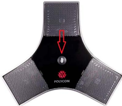
Or by pressing the „microphone-mute button“ on the control display.
